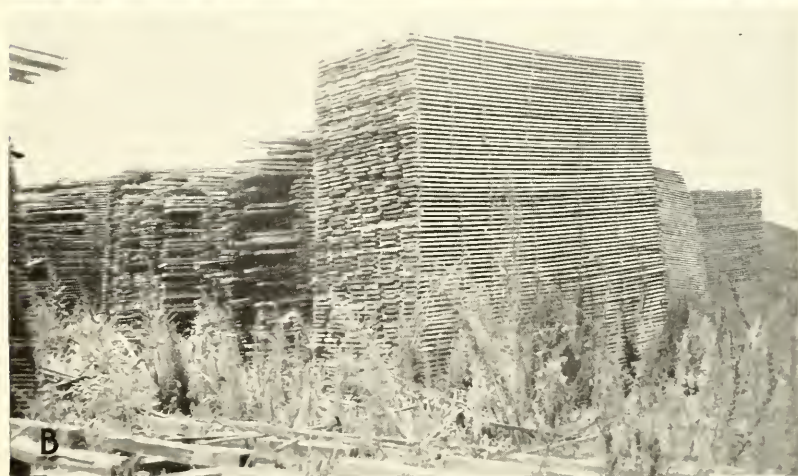
Sanitation in air-seasoning yards: A, Excellent sanitation in an air-seasoning yard; the layout, the foundations, and in the main the piling also are good. All these features are conducive to the necessary good ventilation in the piles; B, poor sanitation in an air-seasoning yard. The loss resulting from stain and decay that are directly chargeable to the choking of circulation caused by the weeds alone would more than pay the cost of putting the yard into good condition and maintaining it properly
